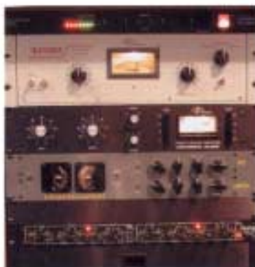
Dynamics processors in regular use at Ironworks include a Universal Audio LA-2A and 1176LN, a Chandler Ltd. TG1, and a Drawmer DS201.
